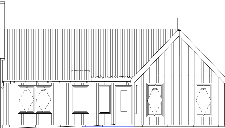
SOUTH ELEVATION HOUSE NO 6
